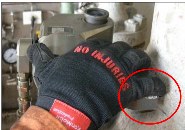
Pinch Point between actuator and spool work
